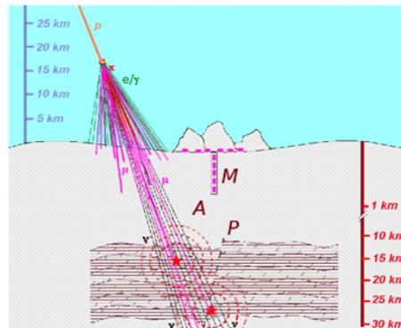
**Fig. 3.** Model of deeper seismic sounding of Earth's crust on the basis of muons from the energetic EAS trunk: P is a deep fault zone; A is elastic vibrations are generated in the seismic stretch environment under local ionization influence from muons passing and propagated as acoustic wave; M is a sensible microphones system.
