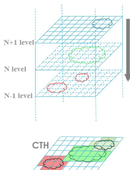
**Figure 1:** Scheme of the algorithm for the CTH determination.
