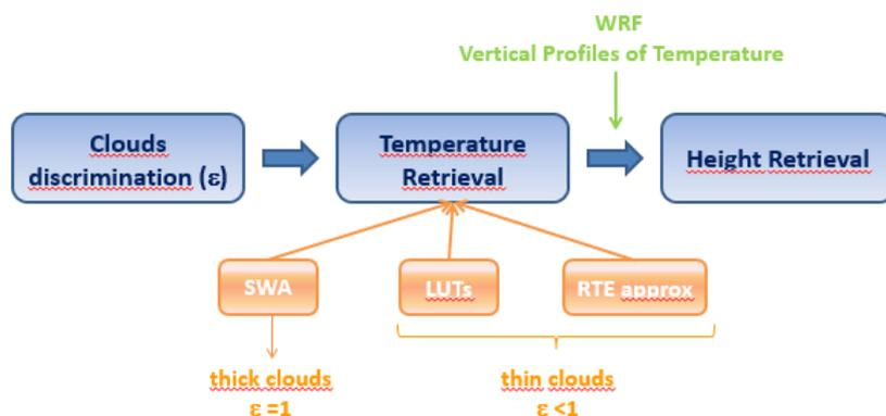
**Figure 3:** Scheme of the radiative method: the measured emissivity allows to calculate a CTT applying different algorithms (Split-Window Algorithm -SWA-, Look Up Tables -LUTs-, Radiative Transfer Equation approximation -RTE approx-) depending on the optical depth and, using the WRF vertical profile, a CTH can be calculated.
