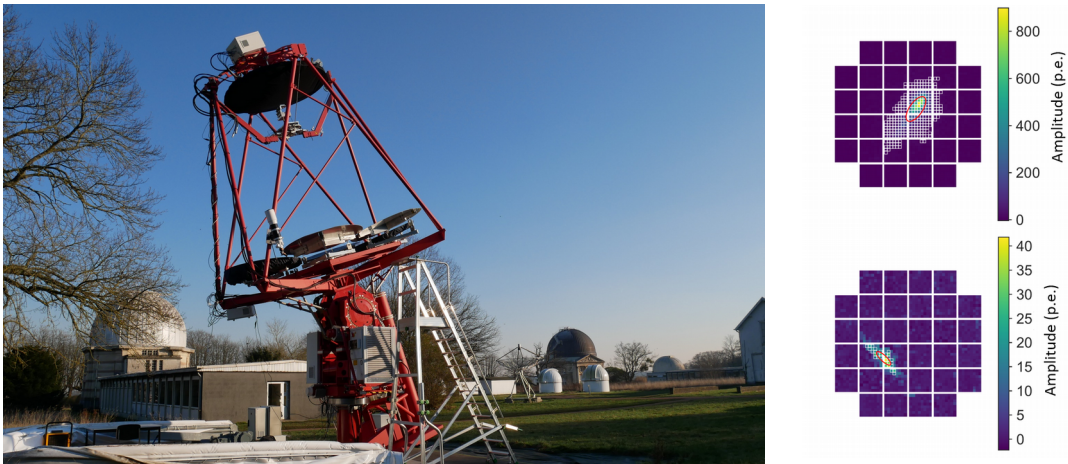
Figure 2: Left: The GCT prototype and its open shelter at the Meudon site of the Paris Observatory during Cherenkov campaigns. The prototype was equipped with two M1 panels out of 6 and the MAPM-based camera of the CHEC team. Right: Examples of Cherenkov events detected by CHEC-M in Meudon. Credit: Observatoire de Paris
