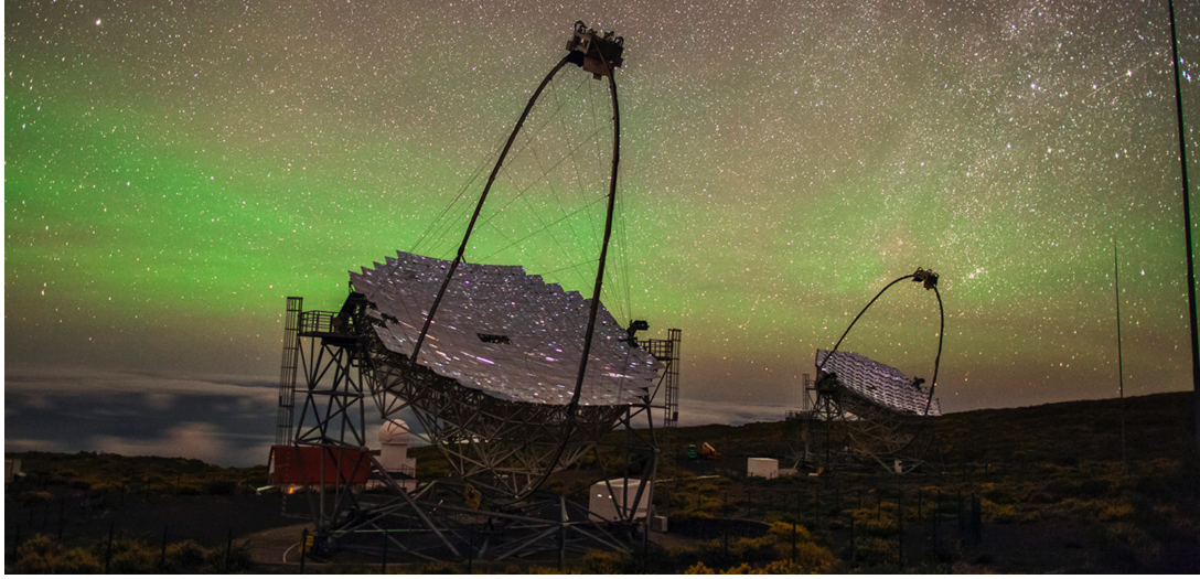
Figure 1: The MAGIC stereo system composed of two 17 m diameter dishes operating simultaneously. Telescopes are located in the Roque de los Muchachos Observatory in the Northern Hemisphere ( 28.7^{\circ}\text{N} , 17.9^{\circ}\text{W} ). Courtesy of D. Lopes (IAC).
