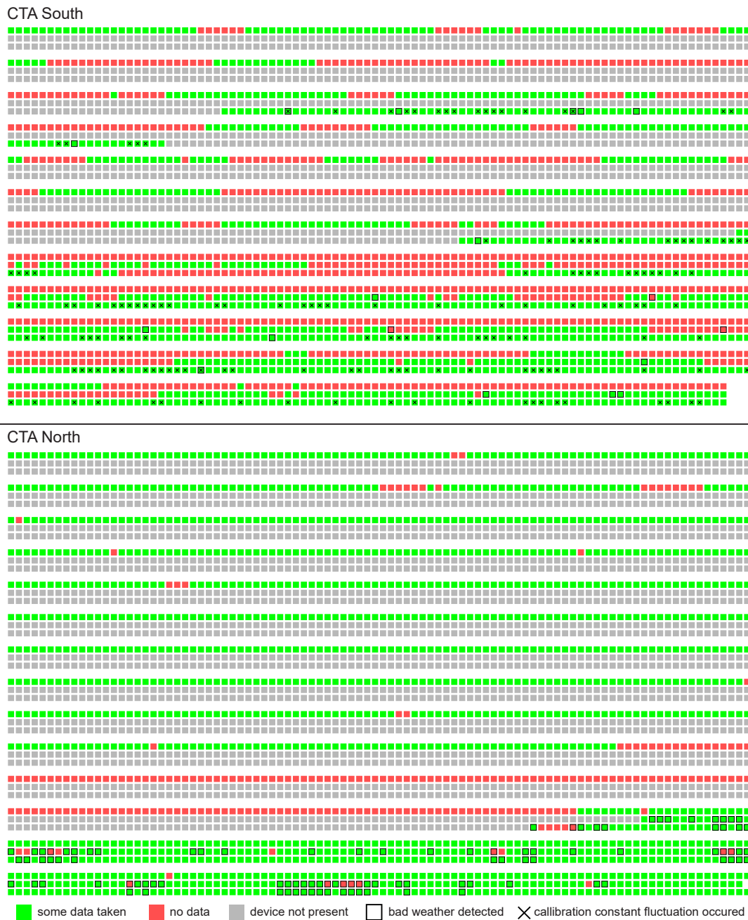
Figure 1: Uptime of the prototype devices at the future CTA sites. In each series, the first line corresponds to the All-sky Camera, the second line to FRAM and the third line to the Sun/Moon Photometer. For CTA South the time period covered is 28/11/2015–26/12/2018, for CTA North it is 15/10/2015–22/05/2019. For each day, the color of the box indicates whether at least some data have been taken, or the instrument was not present at all. It is also shown when the device detectors reported bad weather (rain or high winds) incompatible with device operations, which could be a cause of missing data; in most cases however, the bad weather period did not cover the whole day. For the Sun/Moon Photometer also instances of fluctuating calibration constants are shown; whether the data from these days is recoverable is not clear at the moment.
