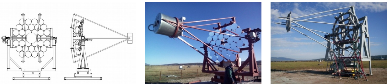
Figure 1: The TAIGA IACT: technical drawing (left), the first IACT (middle) and the second IACT structure (right) in the Tunka valley.
