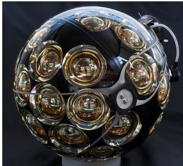
Figure 1: A partial side-view of a KM3NeT Digital Optical Module. The bottom hemisphere, where 19 of the 31 PMTs are located, is oriented to the bottom left of the photo.
