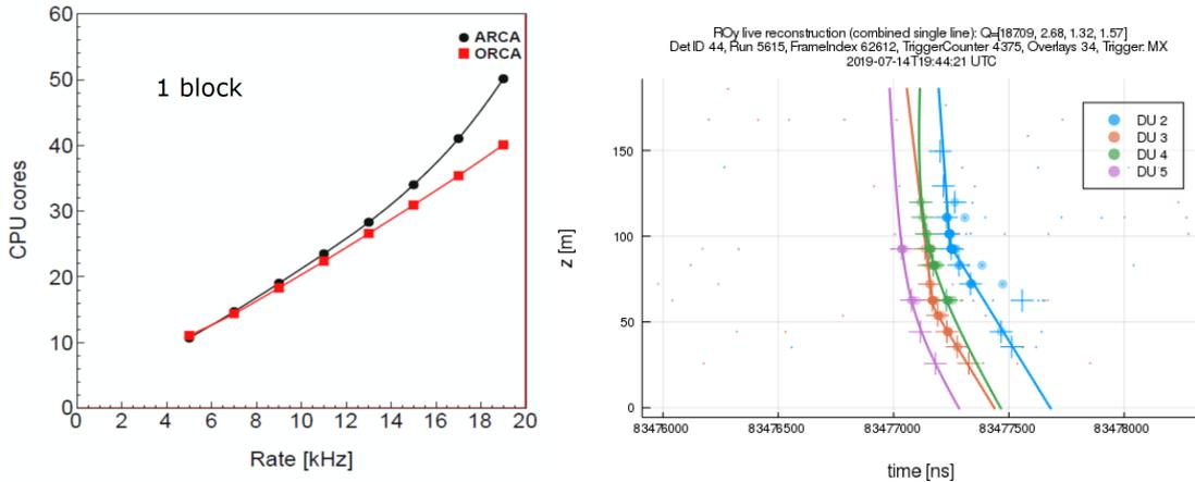
Figure 3: Left: CPU core requirements per building-block vs. PMT single rate; the estimate is obtained by using an Intel® Core™ i5 4570 CPU at 3.20GHz. Right: Example of online monitoring: hit height versus time of the detection and fitted trajectories for the 4-DUs of ORCA .
