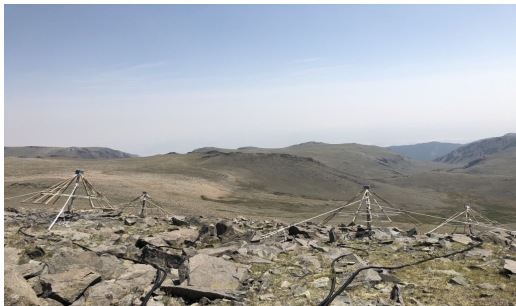
Figure 3: View of BEACON prototype from above the mountain ridge. Antennas were camouflaged to minimize environmental impact.
