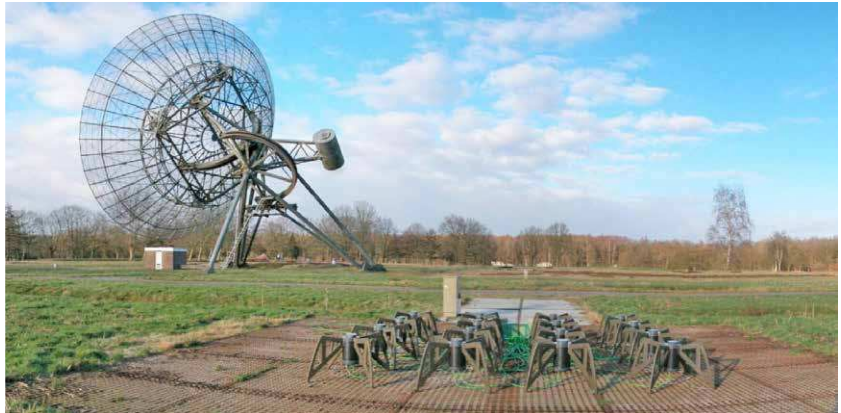
Figure 2: Pre-production prototype of a single LOFAR HBA tile at the WSRT site (excerpt from Panorama picture made by Harm-Jan Stiepel and Adriaan Renting).
