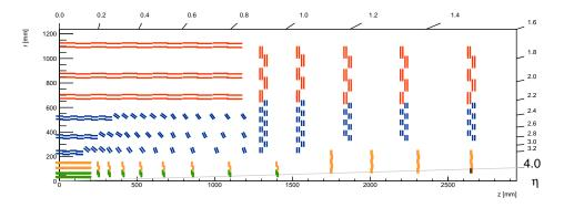
**Figure 1:** Layout of one quarter longitudinal section of the CMS Tracker for the HL-LHC. In green (yellow) the silicon pixel detectors of the Inner Tracker with two (four) readout chips per module. In blue (red) the PS (2S) silicon detector modules of the Outer Tracker (see main text for details).
