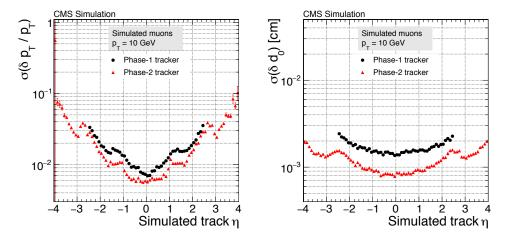
**Figure 6:** Track parameter resolution for the Phase-1 (black dots) and the Phase-2 (red triangles) tracker, from the simulation of single muons with a transverse momentum of 10 GeV. The  $p_{\rm T}$  resolution (left) and the impact parameter resolution (right) show the improved performance of the Phase-2 detector [3].
