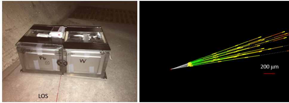
Figure 6: Left: The 30-kg pilot neutrino detector that was installed in the TI18 tunnel in 2018. It collected 12.5 \text{ fb}^{-1} of data. Right: One of vertices found in the detector with no incoming charged track. The vertex axis is compatible with the beam direction.
