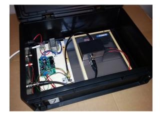
**Figure 1:** Picture of one of the 30 detection modules of the mini-array. The boxes have been home-assembled in the Physics Department of Catania University.
