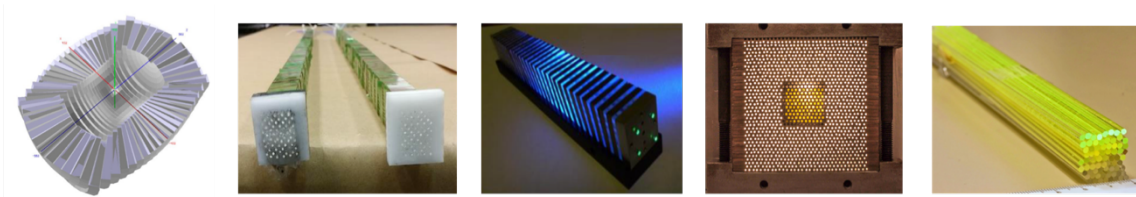
Figure 4: From left to right, IDEA DREAM calorimeter concept and prototype, Shashlik and Spaghetti calorimeter options for LHCb, Homogenous Intelum Time Imaging Calorimeter.
