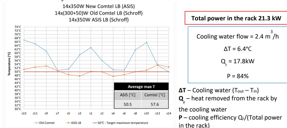
Figure 2. Cooling test results with 350W average per blade.
