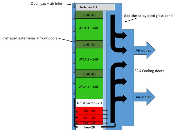
Figure 4. Side view of the 63U ATCA rack with cooling door.
