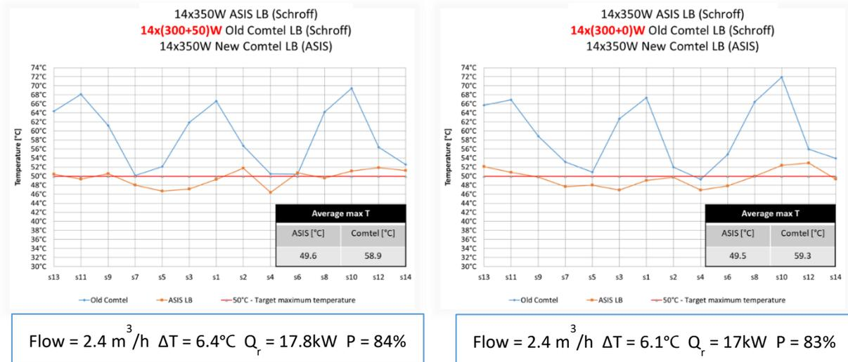
Figure 3. RTM power impact on the cooling efficiency test.
