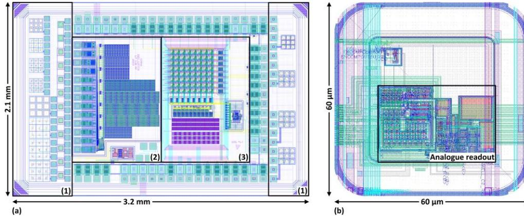
**Figure 7** Layout views: RD50-MPW2 (a) and pixel of the matrix for fast response time (b). Regions (1), (2) and (3) in (a) correspond to the test structures, the peripheral readout electronics and the matrix for fast response times respectively.
