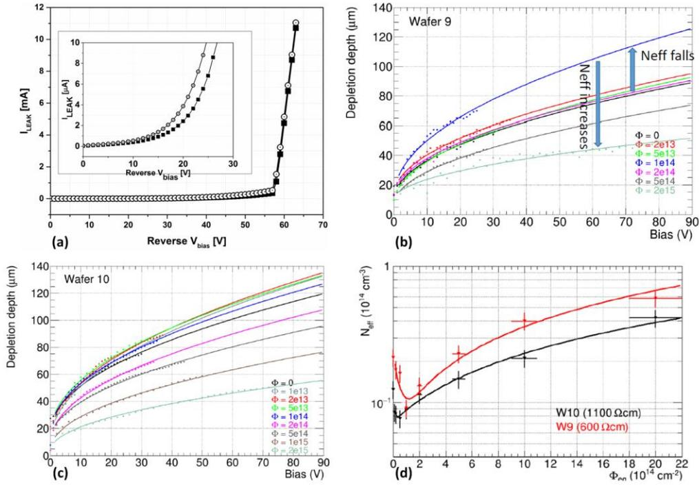
**Figure 4** Performance evaluation of RD50-MPW1: I-V curves of the 600  $\Omega\cdot\text{cm}$  (squares) and 1.1  $\text{k}\Omega\cdot\text{cm}$  (circles) wafers (a), depletion depth before and after neutron irradiation of the 600  $\Omega\cdot\text{cm}$  and 1.1  $\text{k}\Omega\cdot\text{cm}$  (c) wafers [8], and initial doping concentration as a function of 1 MeV neutron equivalent fluences (d) [8].
