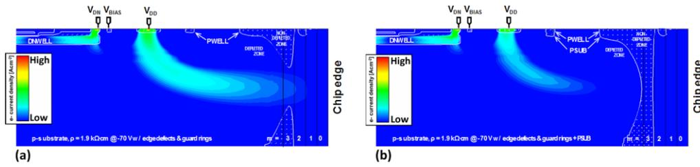
**Figure 6** TCAD simulations of one pixel and the edge of the chip with a guard ring frame: without deep p-well (a) and with deep p-well (b) in the p-type guard rings.
