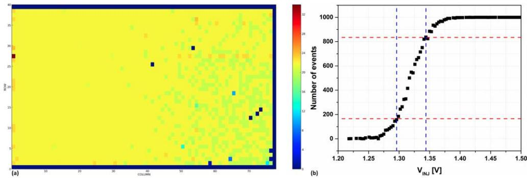
**Figure 5** Performance evaluation of RD50-MPW1: Hit map (a) and S-curve (b).
