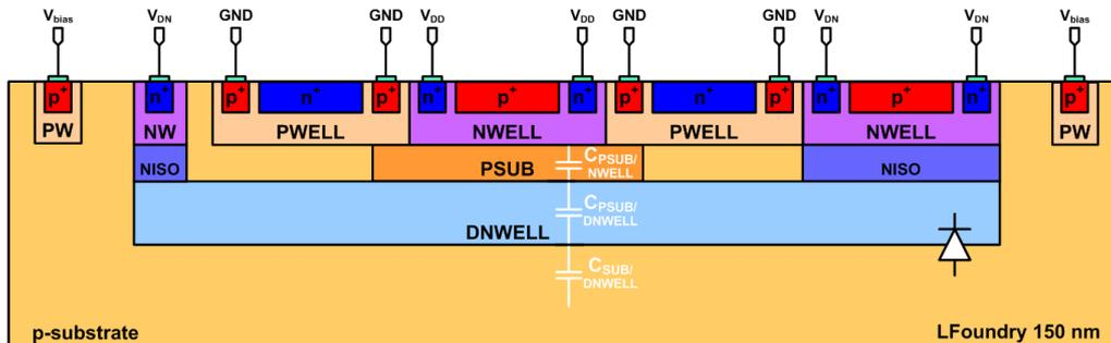
**Figure 2** Schematic cross-section of a pixel in the 150 nm HV-CMOS process from LFoundry. The drawing is not to scale.
