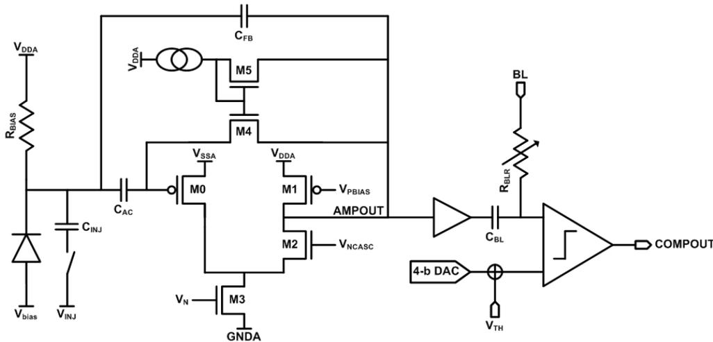
**Figure 3** Schematic of the analog readout electronics of RD50-MPW1.
