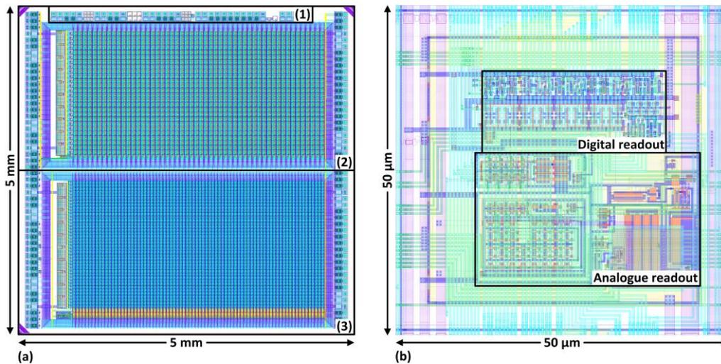
**Figure 1** Layout views: RD50-MPW1 (a) and pixel of the matrix for particle physics experiments (b). Regions (1), (2) and (3) in (a) correspond to the test structures, the matrix for photon counting applications and the matrix for particle physics experiments respectively.
