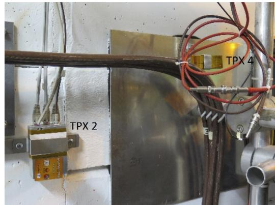
**Figure 5:** TimePix chips installed in MoEDAL.
