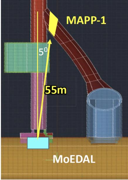
**Figure 10:** Planned positioning of the first phase of the MoEDAL MAPP subdetector, MAPP-1, in the UGC1 gallery, relative to the MoEDAL location as seen from above [98].
