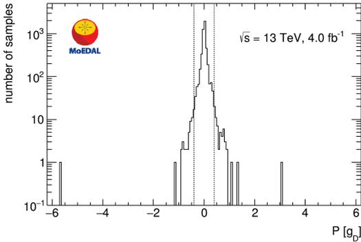
**Figure 6:** SQUID analysis results: Magnetic pole strength (in units of Dirac charge,  $g_D$ ) measured through the induced persistent current in the 2400 aluminium samples of the MoEDAL trapping detectors exposed to 13 TeV  $pp$  collisions in 2015–2017 with every sample scanned twice [56].
