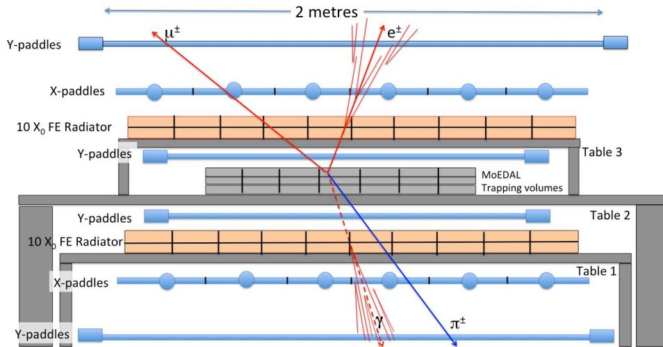
**Figure 12:** The MALL subdetector designed to monitor MoEDAL trapping volumes for the decays of trapped electrically charged particles with lifetimes as long as 10 years [94].
