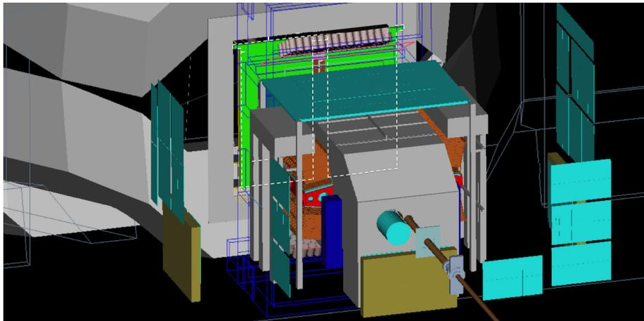
**Figure 1:** GEANT4 visualisation of the MoEDAL experiment around the LHCb VELO region at Point 8 of the LHC prepared with the Panoramix package.
