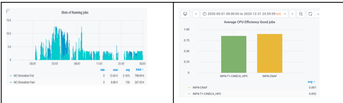
Fig. 2. Left: Job slots used by ATLAS at Marconi A2, from May 2020 to March 2021; Right: Average CPU efficiency of ATLAS jobs running at CINECA compared with job efficiency at INFN-CNAF
