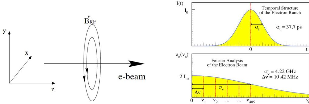
**Figure 5:** Left: magnetic RF-field associated with a bunched e-beam. Right: time structure and corresponding Fourier composition of the LHC bunched beam.
