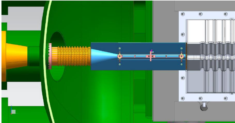
**Figure 4:** Side view of the SMOG2 storage cell system (see text). The beam employed for FT measurements is directed from left to right. The secondary particles move to the right into the VELO detector (light grey).
