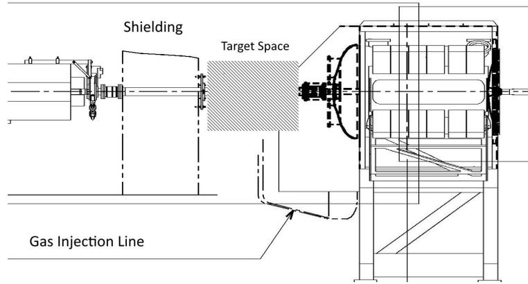
**Figure 7:** View of the region upstream the VELO detector evidencing the space available for the PGT.
