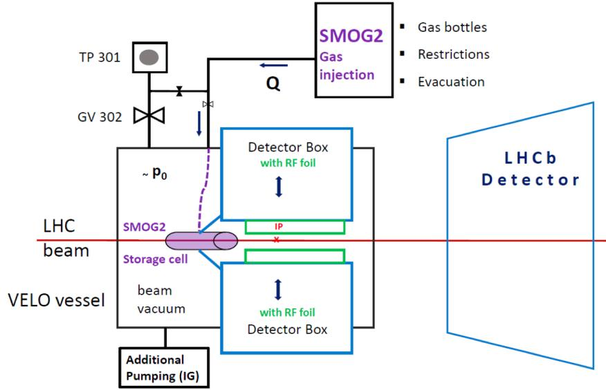
**Figure 3:** Principle of the SMOG2 target (see text). A gas feed system is employed to inject well-defined flow rates which allow for the precise prediction of the target density.
