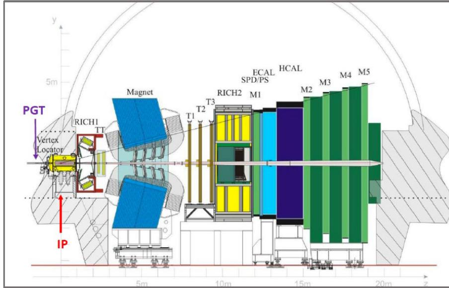
**Figure 2:** Sideview of the LHCb detector. Left: IP8 with VELO and the possible location of the target (PGT).
