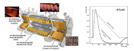
**Figure 1.** (left) Layout of the different subdetectors of the ATLAS Liquid Argon system [2]. The different sections of the calorimeter are labeled, along with their respective absorber materials. Photographs of the hadronic end-cap (HEC), electromagnetic barrel (EMB) and forward (FCal) calorimeters are overlaid [3]. (right) Overlap of the triangular ionization signal collected directly by the electrodes and the reconstructed signal after the shaper and sampler.
