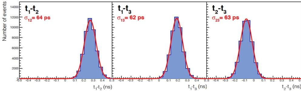
**Figure 2:** Distributions of time differences between pairs of ETROC1+LGAD layers from the three-layered telescope used at FNAL test beam.
