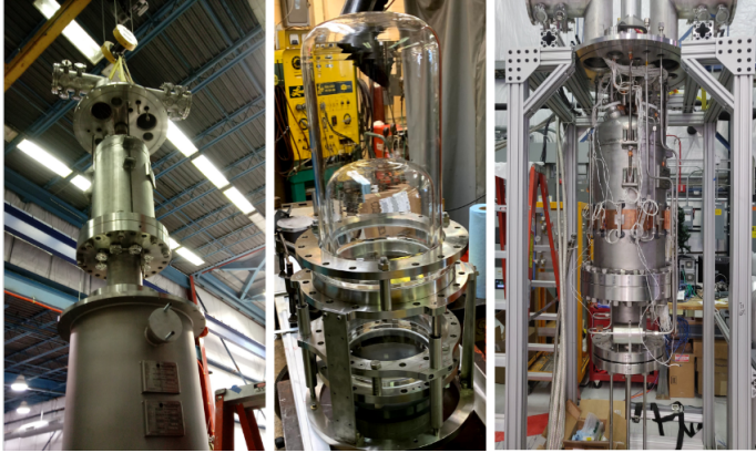
Figure 5: Pressure vessel (PV) inside the vacuum jacket for pressure test (left); Jar arrangement with its bellow system (middle); Wiring of various sensors around PV and connections of the cooling lines to the PV (right).
