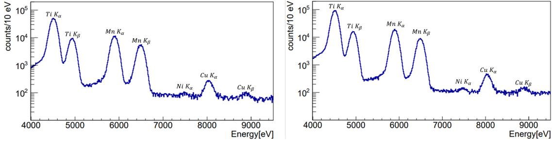
**Figure 1:** Spectra collected with partial shielding configuration (only lateral part). On the left, with 100 A circulating on target; On the right, without current. In the spectra, titanium and manganese lines come from the Fe-55 radioactive source installed in the apparatus for calibration; the nickel line comes from the detectors’ ceramic support.
