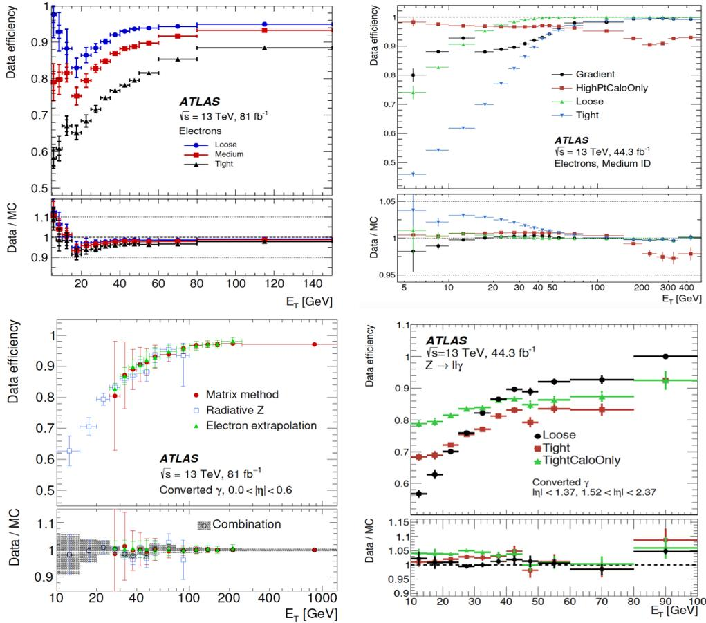
**Figure 3:** ID efficiency on the left and isolation efficiency on the right for various WPs in ATLAS. Top plots are for electrons and bottom for photons. Top panel of the plots show the efficiency in data, whereas, bottom panel shows the estimated data/simulation scale factors. The uncertainties include quadrature sum of statistical and systematic uncertainties.
