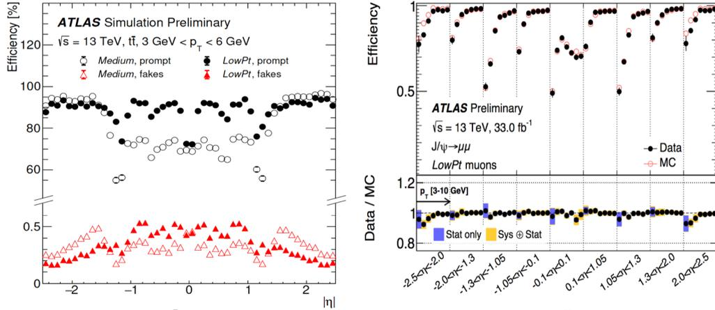
**Figure 5:** Left plot shows the low  $p_T$  muon ID efficiency in simulation showing a gain in efficiency for low  $p_T$  muons especially in the barrel. The efficiency is close to 90% whereas the mis-identification rate is below 0.5%. Right plot shows the estimated efficiency in data as a function of  $p_T$  in various  $\eta$  bins. It can be seen that the SFs are very close to 1. These plots are for the ATLAS detector.
