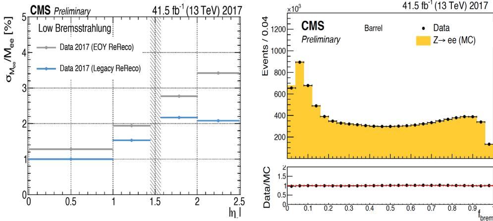
**Figure 1:** Comparison of di-electron mass resolution from "Legacy ReReco" to that in the "EOY ReReco" is shown on the left. There is more than 40% improvement in the resolution in the highest  $\eta$  bin. Distribution of the fraction of the momentum lost by bremsstrahlung between the inner and outer parts of the tracker for electrons from  $Z$ -boson decays in the ECAL barrel in the "Legacy ReReco" dataset is shown on the right.
