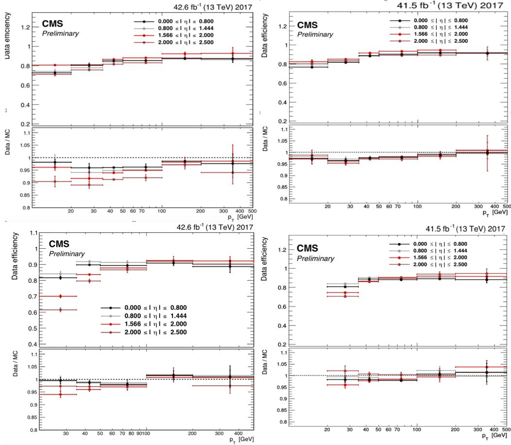
**Figure 2:** Electron ID efficiency for MVA ID with WP of 90% on the top and photon loose ID efficiency on the bottom. Left plot is for the EOY ReReco, right plot is for the Legacy ReReco for CMS. Top panel of the plots shows the efficiency in data, whereas, bottom panel shows the estimated data/simulation scale factors. It can be seen that the SFs are much closer to 1 in the Legacy ReReco dataset. The uncertainties include quadrature sum of statistical and systematic uncertainties.
