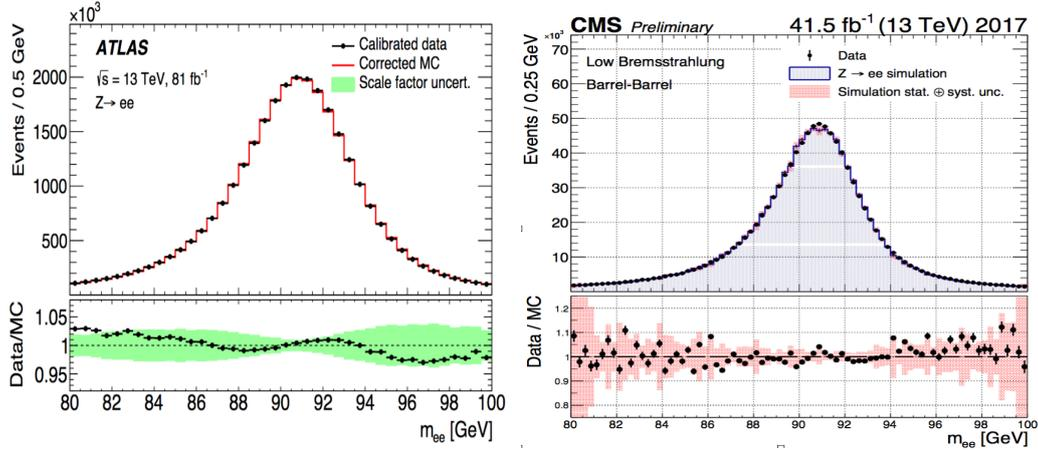
**Figure 4:** Invariant mass distribution of  $M_{ee}$  after the scale corrections in data and smearing corrections in simulation. Left is for ATLAS and right is for CMS.
