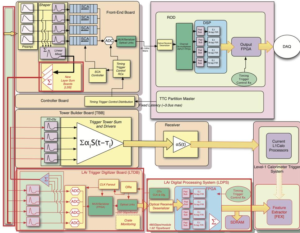
**Figure 1:** Schematic block diagram of LAr calorimeters' readout electronics after the Phase-I upgrade. The new components are indicated in red [3].
