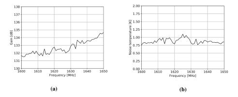
Figure 4: (a) Total gain and (b) system noise temperature of the CAPP-8TB receiver chain.
