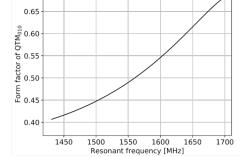
Figure 2: Form factor of QTM<sub>010</sub> mode.
