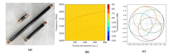
**Figure 1:** (a) CFRP tubes. (b) Mode map of the cavity with frequency tuning mechanism, lines denote  $QTM_{010}$  (lower) and  $QTM_{011}$  (upper) modes respectively. (c) Typical Smith chart of reflection coefficient from the strong antenna.
