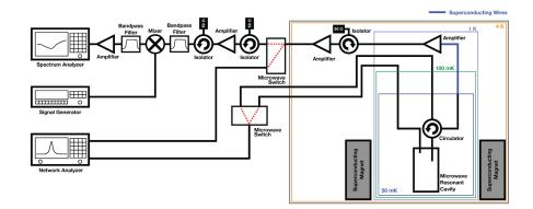
Figure 3: Schematics of the entire receiver chain in the CAPP-8TB experiment.
