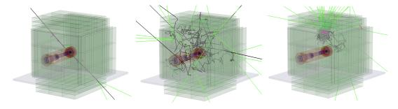
**Figure 3:** *Geant4* Monte Carlo simulations of the detector, shielding VETO systems using RESTSoft [19]. From left to right, a simulated muon, neutron and high-energy gamma. Green lines describe the trajectories of gammas and black lines of neutrons).
