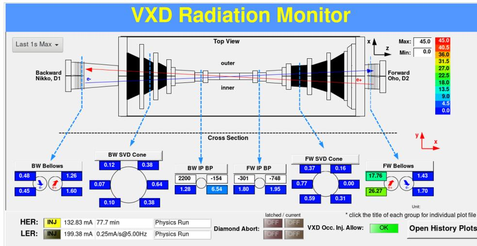
**Figure 1:** On-line interface: a real-time monitor of radiation for accelerator operators. On this interface, several options for dose rates are provided: the original 10 Hz values, the average of 1 s, the maximum in 1 s, the average of 100 s, and the average of 1000 s.
