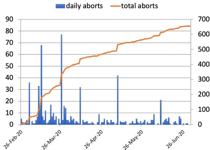
**Figure 3:** Statistics of diamond aborts during the 2020 running until July 1st. During machine studies, the frequency of aborts triggered by the diamond system is  $\sim 10$  /hour, while the frequency decreases to  $\sim 1$  to 2 /day during physics data taking.
