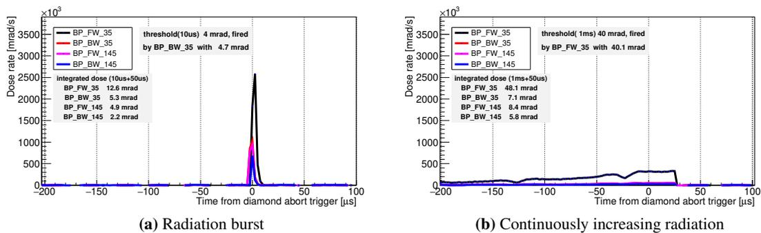
**Figure 2:** Examples of the two types of aborts. The first type (a) is configured to cope with radiation bursts which have spikes-like shape. While the second type (b) is responsible for continuously increasing radiation in the shape of growing tails. Doses integrated within the corresponding time window of each sensor are calculated and the sensor whose dose exceeds the threshold is highlighted.
