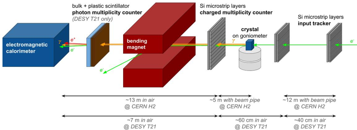
**Figure 1:** Experimental setup for the study of SF-related radiation processes by electrons impinging on oriented crystalline samples. Details are given in the text body.
