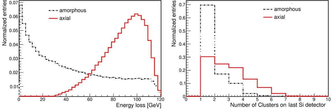
**Figure 2:** Results of the 2017 beamtest of the SF regime in [001]-axially oriented  $\text{PbWO}_4$ . Energy loss inside the crystalline sample (left, adapted from [1]) and output charged particle multiplicity measured by the downstream silicon microstrip layers (right) in random and axial angular orientations.
