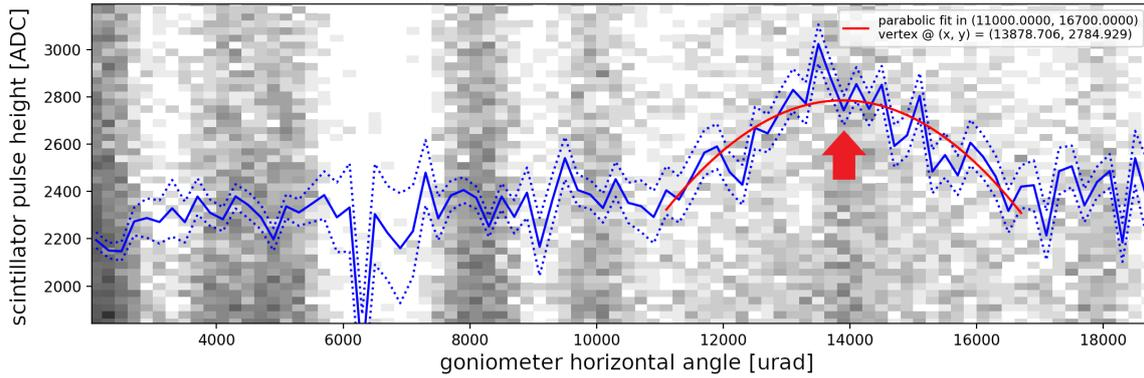
**Figure 3:** Response of the downstream photon counter installed in the DESY 2019 setup as a function of the relative alignment of a [100]-axially oriented thin  $\text{PbWO}_4$  sample. The axis position, which features a strong enhancement in the detector mean signal, is highlighted with a red arrow.
