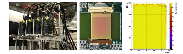
**Figure 2:** The MuPix Telescope (left) and MuPix8 chip (middle) used for the test-beam at PSI with the resultant measured hit efficiency of the sensor (right).
