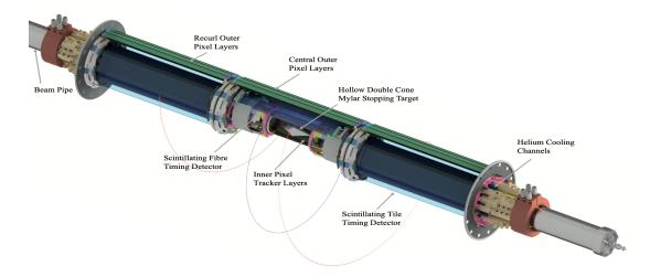
Figure 1: Illustration view of the active configuration of the Mu3e detector.
