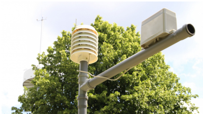
Figure 1: MESSI with attached tipping bucket rain gauge to collect precipitation, Photo: Andreas Trojand. This work is licensed under a Creative Commons Attribution-NonCommercial-NoDerivs 3.0 Germany (CC BY-NC-ND 3.0 DE) License .
