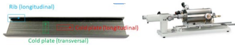
Fig. 5 Set-up used for the specimens CTE measure
