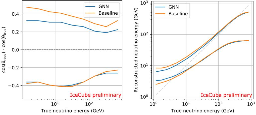
**Figure 4:** Bands comparing the resolution vs energy of our GNN with the baseline algorithm, for the zenith angle  $\cos(\theta)$  (left) and the neutrino energy  $E$  (right). 68% of the best reconstructed events lie between the plotted bands. The dashed lines indicate the target values.
