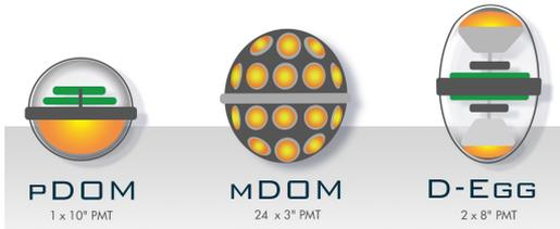
**Figure 2:** New DOM architectures for the Upgrade strings.
