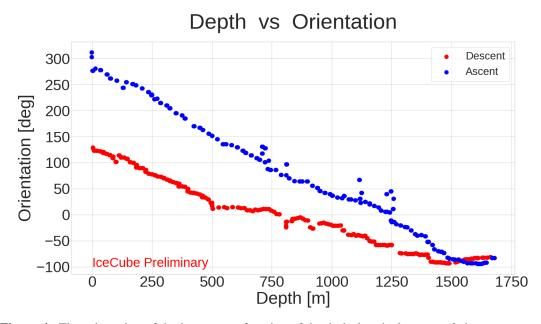
**Figure 4:** The orientation of the logger as a function of depth during deployment. 0 degrees were chosen arbitrarily and this plot serves to show the amount of rotation during deployment.
