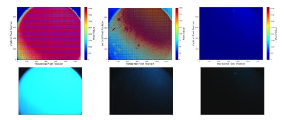
**Figure 3:** Images captured with the camera at various depths. From left to right pictures taken at 810 m, 1250 m and 1610 m are shown. The top row shows false color plots of the image data and the bottom row are true color images. All images use the same settings and while the LED was shining. The corners of the images are not illuminated due to the size of the lens and the image sensor. The images at 1250m show the flakes in the estisol very clearly.
