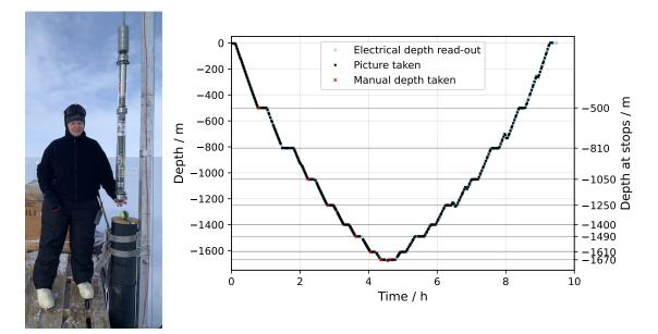
**Figure 2:** Left: Photo taken at the SPICEcore hole with the logger prior to deployment. Right: The logger depth during deployment as a function of time. Green lines mark the stops during ascent and descent.
