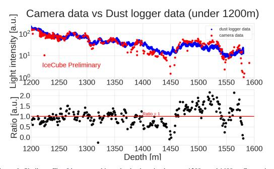
**Figure 6:** Similar to Fig. 5 but zoomed in to the depth region between 1200m and 1600m. Comparison of the dust logger and the camera brightness data as a function of depth. In the lower part the ratio of camera and dust logger brightness is shown.
