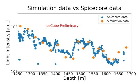
**Figure 7:** A comparison of simulated images generated with the PPC simulation package. The simulation was based on the current IceCube South Pole ice (SPICE) model [3]. Depth values were adjusted to account for the tilt in the ice layers based on measurements with the dust logger at the IceCube site and the SPICEcore. There is an uncertainty of 30 m to the depth values of the simulation due to the tilt of the ice layers between the SPICEcore hole and the IceCube site.
