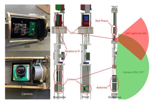
**Figure 1:** Photos and 3D diagrams of the camera and LED inside the luminescence logger from different viewing angles. The position of the camera and the LED board are highlighted. The field of view of the camera and the LED light cone are shown.
