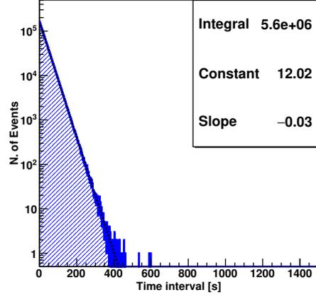
**Figure 3:** Distribution of normalized time delay between triggers of the last run. The exponential fit shows that the stochastic time serie is well in agreement with the expected Poisson statistics.
