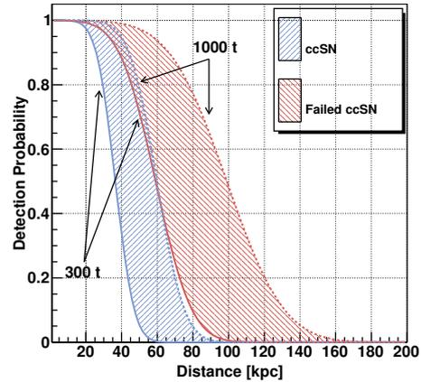
**Figure 5:** LVD detection probability versus source distance for the  $F_{im} = 1/100 \text{ year}^{-1}$  for both ccSN and fSN in the range of minimum (300 t) and maximum (1000 t) allowed active mass.
