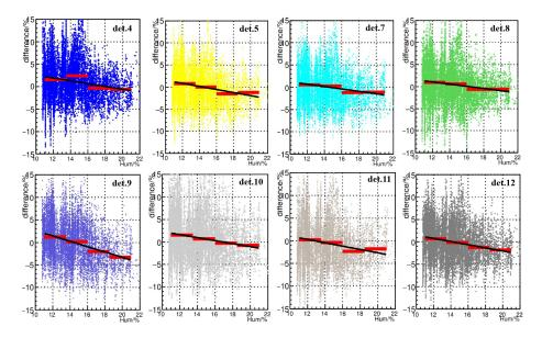
**Figure 3:** linear fitting of profile of  $\delta$  vs humidity of No.1 soil moisture meter
