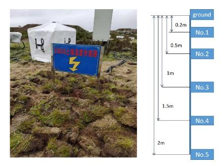
**Figure 2:** Configuration of soil moisture meters.
