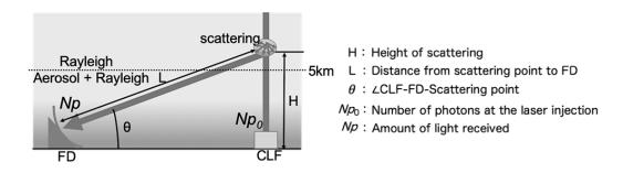
Figure 3: Overview of the laser path in the analysis.
