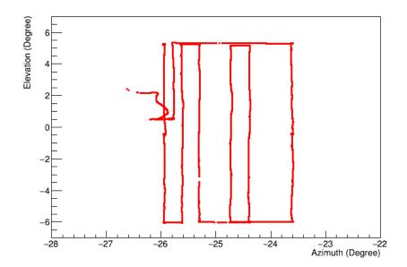
**Figure 4:** First drone pulser flight path recorded by DGPS. The elevation angle is  $0^{\circ}$  in horizontal direction, and azimuth angle is defined as  $0^{\circ}$  at geographic east and positive to north, where antennas point to  $\sim -27^{\circ}$ .
