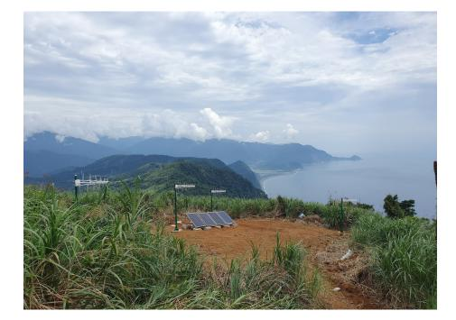
Figure 2: TAROGE-4 station, LPDA antennas pointing horizontally to ocean.
