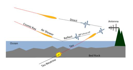
Figure 1: The detection concept of TAROGE, Adapted from [4].
