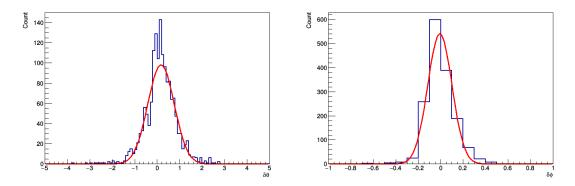
Figure 5: Angular resolution in elevation (Left) and azimuth (Right).
