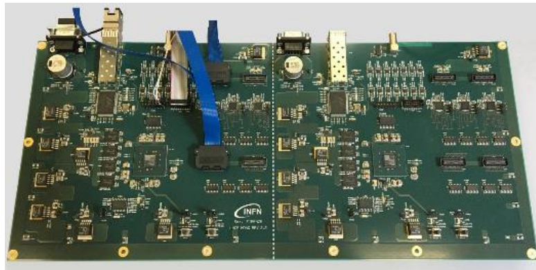
Figure 4: A photo of new MDAQ board. Analog signals transferred from PACE 3 chips are digitized in this board located near the Arm2 detector, and the data is sent to a counting room via 1 Gbps optical link with TCP/IP protocol.
