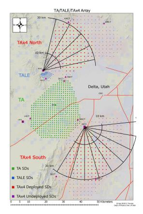
**Figure 1:** Map of the entire TA experiment. The magenta triangles are locations of communication towers and the magenta squares are FD sites. The 257 deployed TAx4 SDs are shown as red circle to the northeast and southeast. While the purple circles are planned location of the remaining 243 TAx4 SDs to be deployed. The 2 fan shapes drawn with black lines show the field of view of TAx4 FDs.
