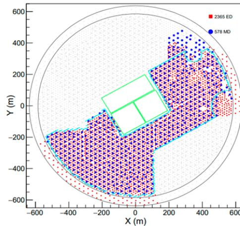
**Figure 1:** The layout of half array of LHAASO-KM2A [8]
