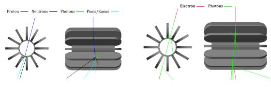
**Figure 4:** 10 GV proton Geant4 simulation event. The detectors shown in Fig. 3 are present in the simulation, but not shown in the event display.
