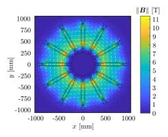
**Figure 1:** The magnetic flux density *B* on the surface of the ARCOS magnet that consists of 12 racetrack-shaped double-pancake coils.
