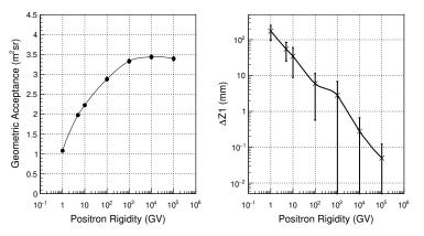
**Figure 9:** Left: Positron rigidity acceptance. Right: The corresponding deflection  $\Delta Z1$  across the entry side field region. The quoted errors represent the RMS variation of the average value of the  $\Delta Z1$  distributions.
