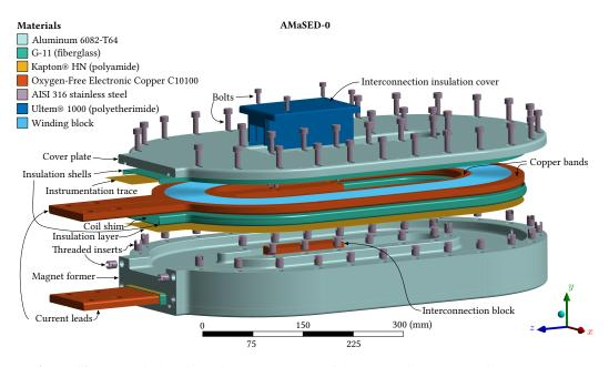
Figure 12: An exploded view of the components of the mechanical model coil, AMaSED-0.
