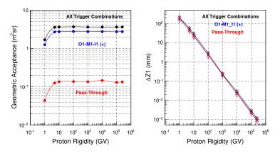
**Figure 8:** Left: Proton rigidity acceptance. Right: The corresponding deflection  $\Delta Z1$  across the entry side field region. The quoted errors represent the RMS variation of the average value of the  $\Delta Z1$  distributions.
