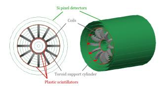
**Figure 3:** On the left: a cross-sectional view of the silicon pixel detector planes (green), plastic scintillator planes (red), toroidal coils and cylindrical support structure (gray). On the right: A three-dimensional view.
