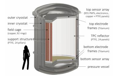
Figure 1: Possible realisation of the DARWIN TPC equipped with 3-inch PMTs inside the cryostat.
