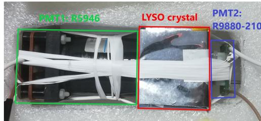
**Figure 3:** LYSO set up for calibration purposes
