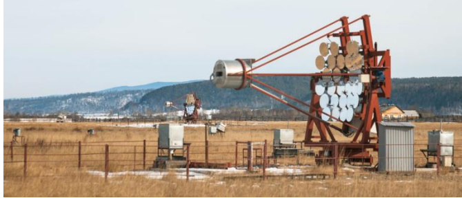
Figure 2. The two Imaging Atmospheric Cherenkov Telescopes of the TAIGA-IACT array.
