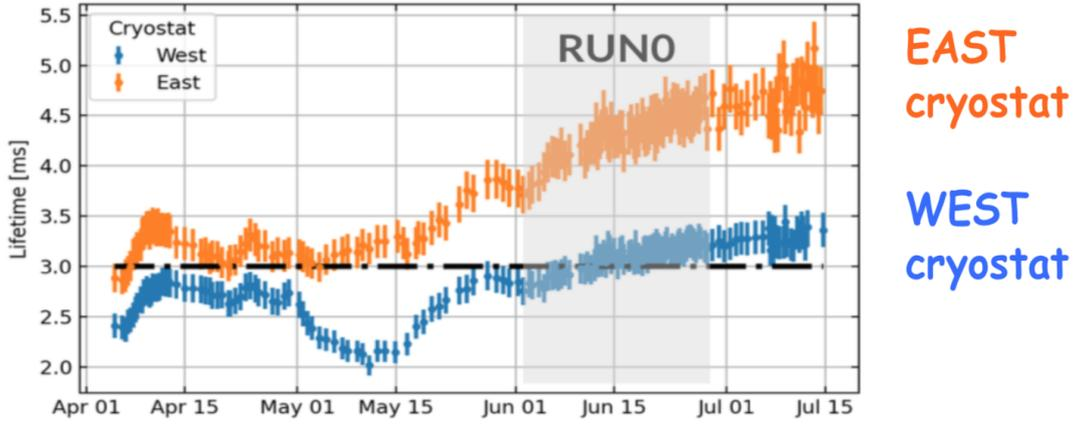
**Figure 3:** Evolution of ICARUS electron lifetime from April to July 2021. East cryostat in orange, West in blue.
