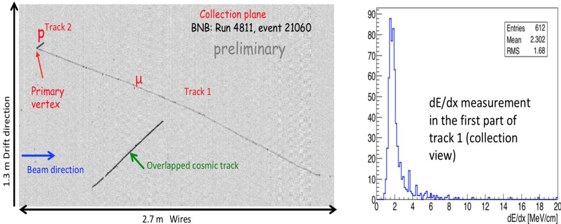
**Figure 4:** A  $\nu_\mu$  CC interaction of a BNB neutrino in ICARUS. On the left, the 2D projection on the Collection plane is shown: Track 1 is a stopping muon candidate, with length  $\sim 2.8$  m and  $E_{dep} \sim 650$  MeV, while Track 2 is likely a proton with length  $\sim 11$  cm and  $E_{dep} \sim 100$  MeV. The plot on the right shows the  $dE/dx$  distribution in the first 2 m of the muon, compatible with expectations for a single MIP.
