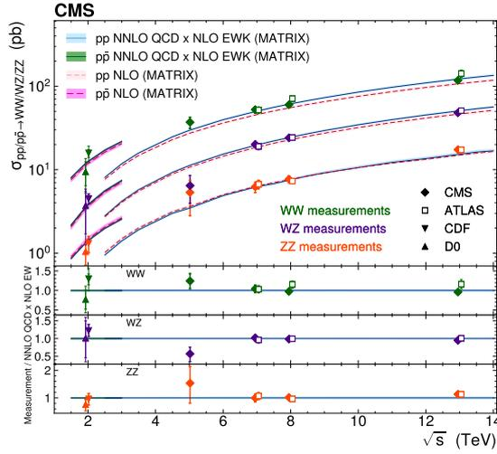
**Figure 1:** Results obtained in this analysis and other diboson production cross section measurements at different center-of-mass energies for the CMS, ATLAS, CDF, and D0 Collaborations are presented, and compared with the NNLO QCD×NLO EW and NLO predictions from MATRIX [5]. The vertical error bars represent the uncertainty in the measured cross section. [1]
