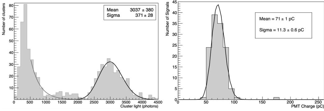
**Figure 1:** Distribution of the light (left) and charge (right) yield for collected respectively with the sCOMS sensor and PMT by exposing the LEMON detector to a  $^{55}\text{Fe}$  X-ray source.
