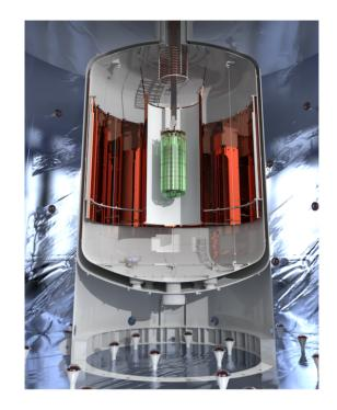
**Figure 1:** Detector systems positioned in the center of the LAr cryostat equipped with wavelength-shifting reflectors. The cryostat is placed in a water tank instrumented with photomultipliers and used as a Cherenkov muon detector.
