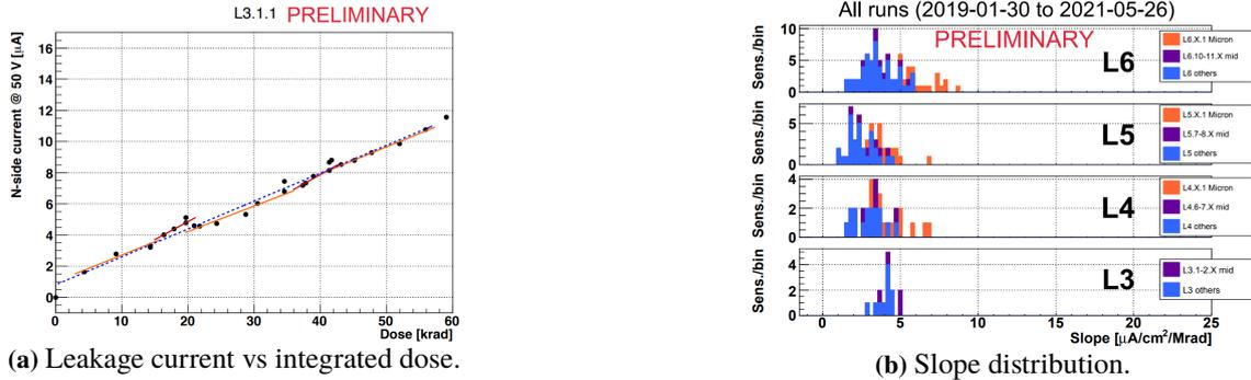
**Figure 3:** (a) Leakage current in one forward sensor of layer-3 as a function of the integrated dose. The red lines are the linear fitting results for each Belle II operation period, and the blue dotted line is the linear fitting result over 2.5 years of operation. (b) Distributions of slopes of the linear fitting results for all sensors in the four layers.
