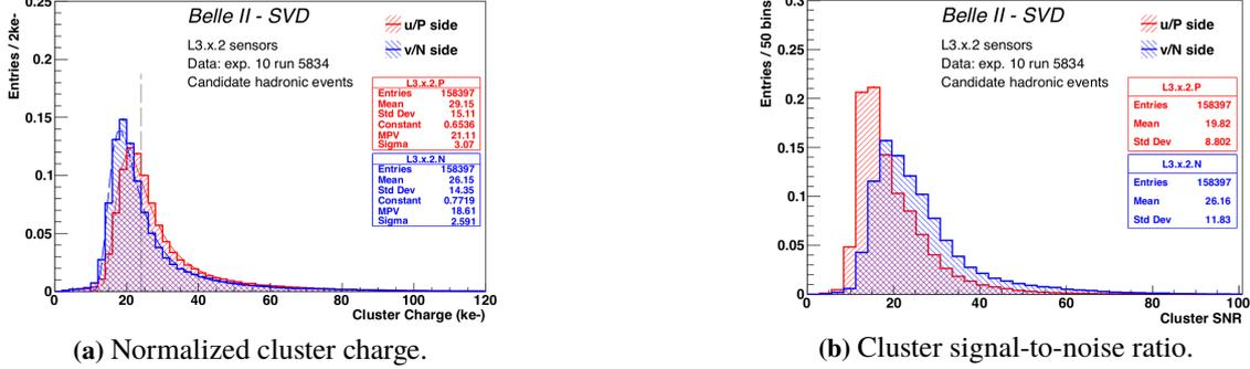
**Figure 2:** Distributions of the cluster charge normalized with the track path length and scaled to the sensor thickness  $320 \mu m$  (a) and the cluster signal-to-noise ratio (b) of one sensor in layer-3. The red and blue distributions correspond to the  $p$ - and  $n$ -side, respectively. The dashed grey line in correspondence of  $24 ke^-$  in plot (a) represents the expected most probable value of the MIP.
