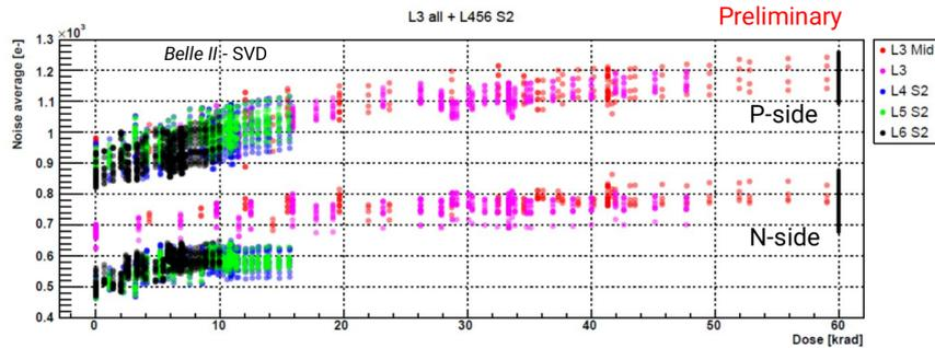
**Figure 4:** Averaged noise as functions of the integrated dose for layer-3 middle-plane sensors, the remaining layer-3 sensors, and one middle sensor of layer-4, 5 and 6.
