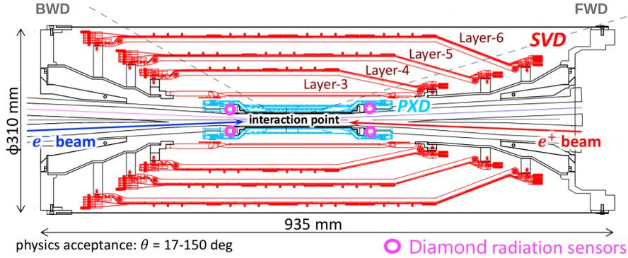
**Figure 1:** The cross-section view of the VXD: SVD and PXD are represented with red and light blue color, respectively. The pink circles indicate the positions of the diamond sensors installed on the beam pipe.
