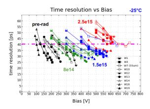
**Figure 2:** Time resolution as a function of the bias voltage of ETL LGAD sensors produced by FBK. Each color defines an irradiation fluence: (black) new sensors; (green)  $8 \cdot 10^{14} n_{eq}/cm^2$ ; (blue)  $1.5 \cdot 10^{15} n_{eq}/cm^2$ ; (red)  $2.5 \cdot 10^{15} n_{eq}/cm^2$ . Taken from [7].
