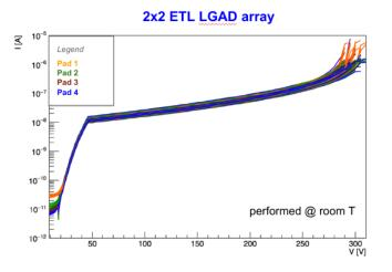
**Figure 1:** IV curves of the four pads of 2x2 arrays from the latest LGAD production by FBK, UFSD3.2 [5].
