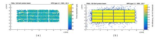
**Figure 3:** Beam test results on the time resolution (a) and hit efficiency (b) uniformity of a 4×4 LGAD array from the HPK3.1 production. Measurements performed at the Fermilab Test Beam Facility. Taken from [8].
